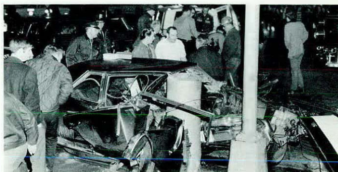
This solid barrier put up by the city of Aberdeen (13 inches from this curved roadway) to protect a breakaway light pole caused two deaths and a $214,000 verdict against The City, Breivo v. Aberdeen , 15 Wn App 520 (1976).
